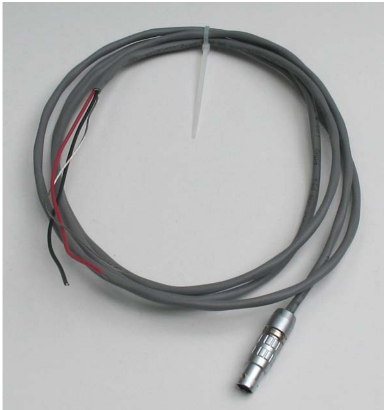
Figure B4. Power cable from RibEye trunk box
