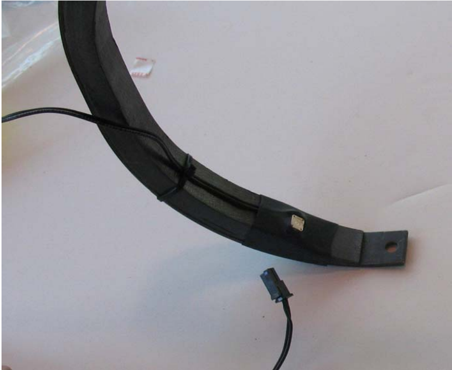
Figure 24. Flat LED and lead wire installed
