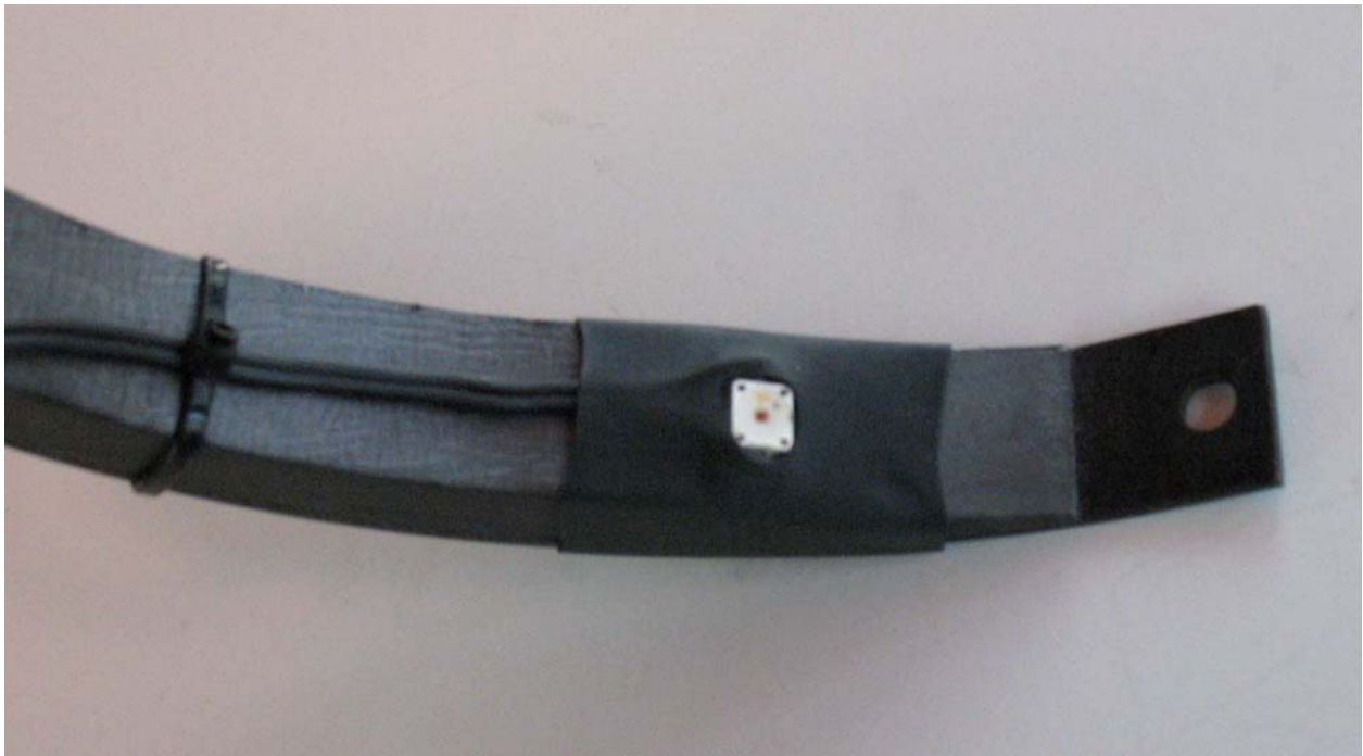
Figure 22. Flat LED in place after heat-shrinking
