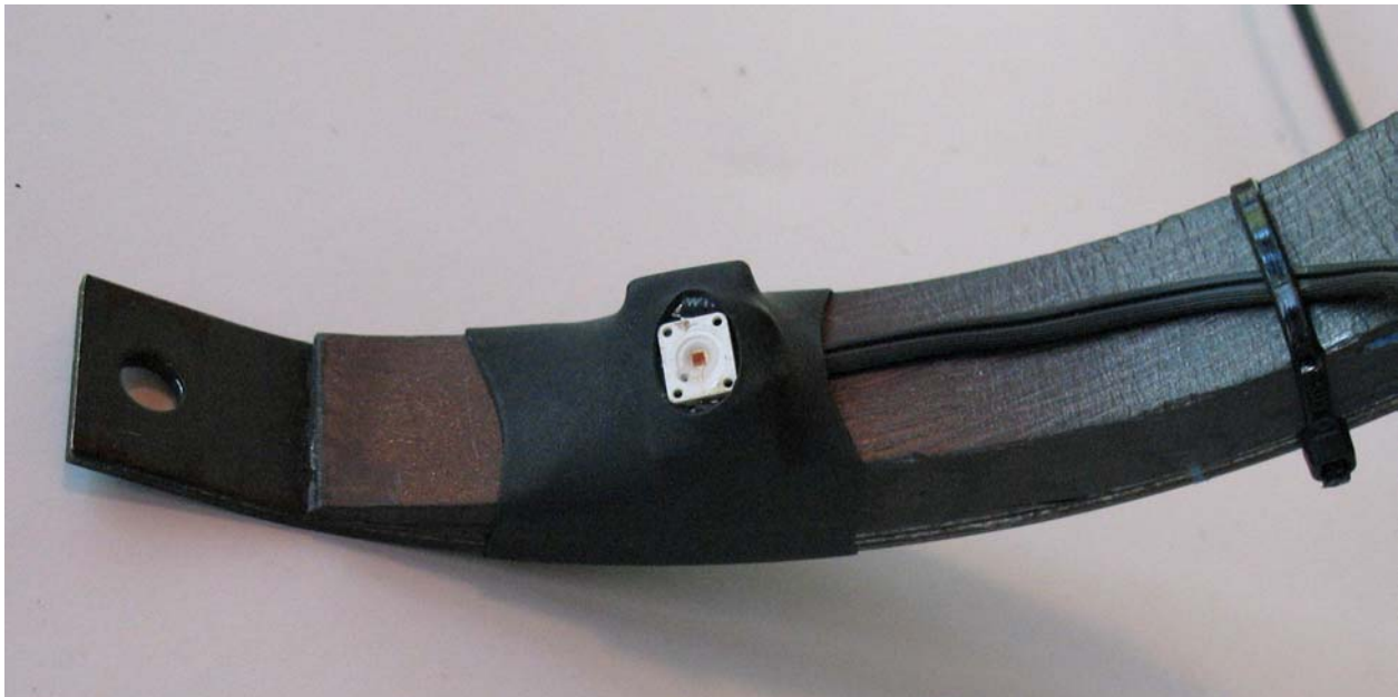
Figure 23. Angled LED in place after heat-shrinking
