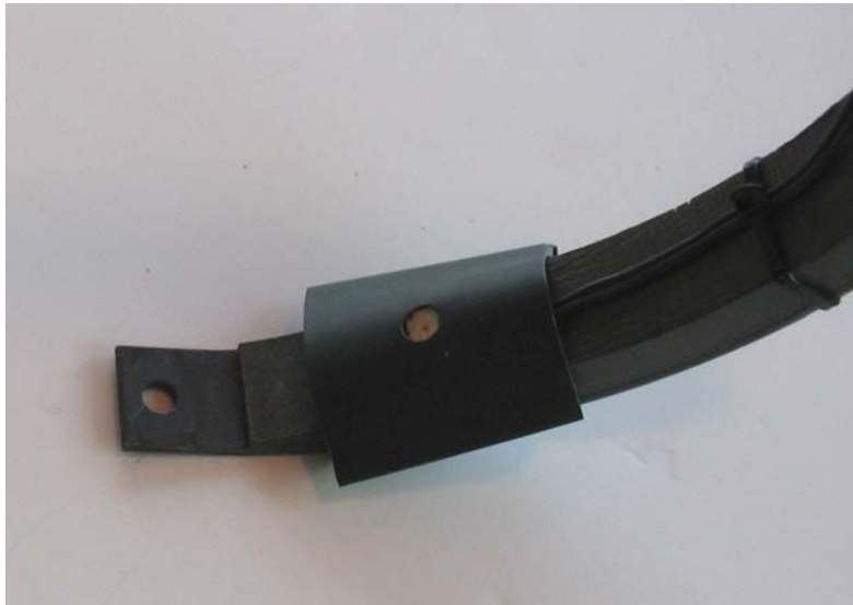
Figure 20. Heat-shrink sleeve in place over angled LED
