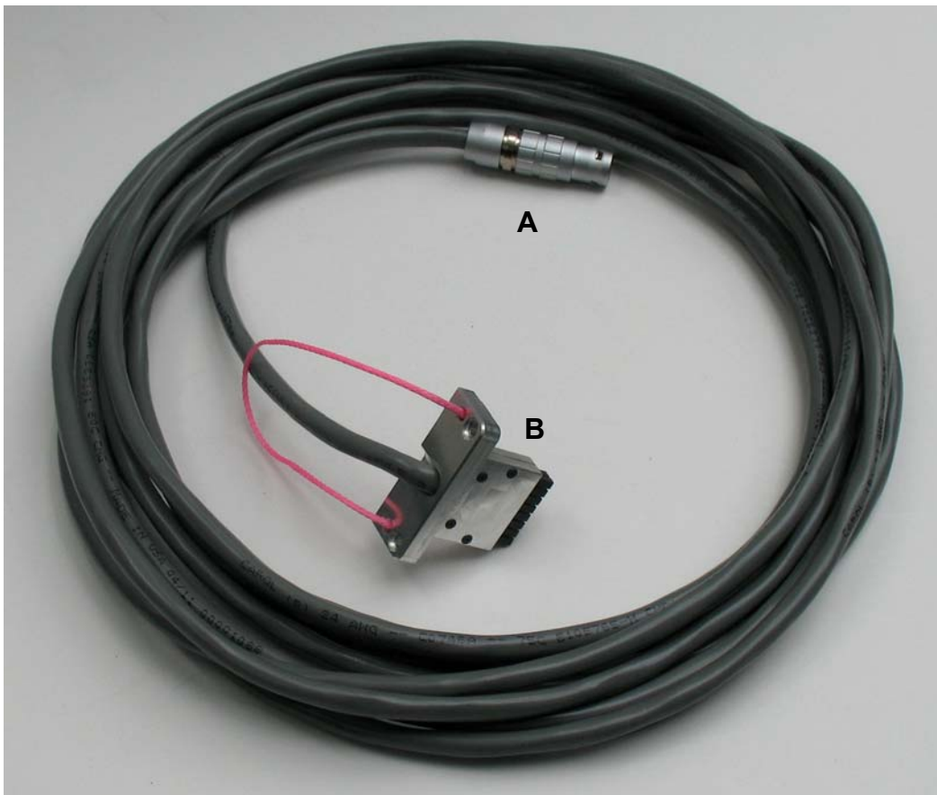
Figure B1. RibEye controller cable and connector A = Souriau end; B = Microfit end (connector)
