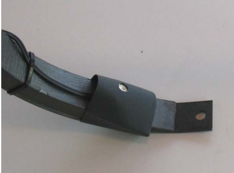
Figure 20. Heat-shrink sleeve in place over angled LED
