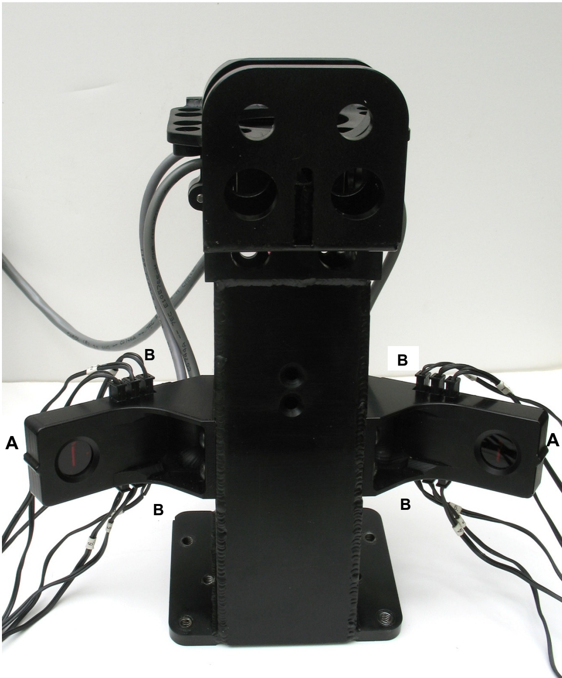
Figure 2. Front view of spine A = sensor heads; B = LED connector blocks
