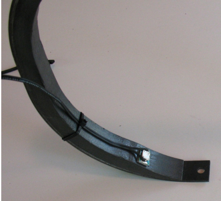
Figure 17. Flat LED in place on rib with lead wire secured by nylon tie
