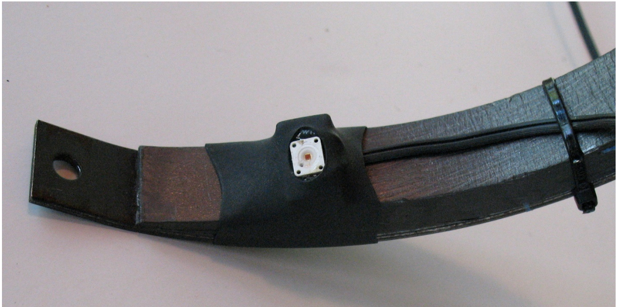
Figure 23. Angled LED in place after heat-shrinking
