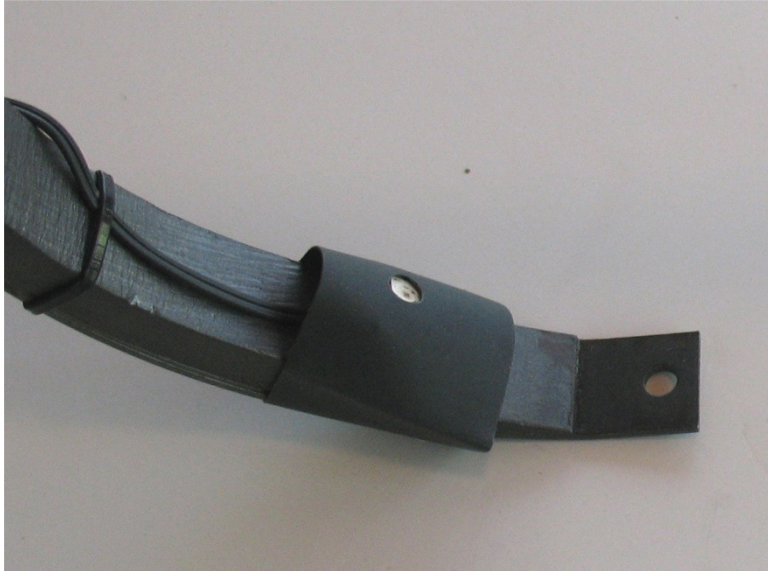
Figure 20. Heat-shrink sleeve in place over angled LED
