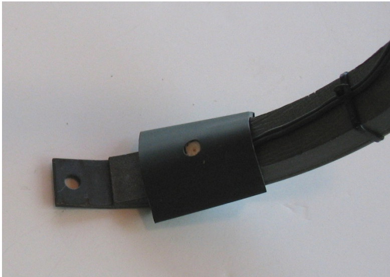
Figure 20. Heat-shrink sleeve in place over angled LED
