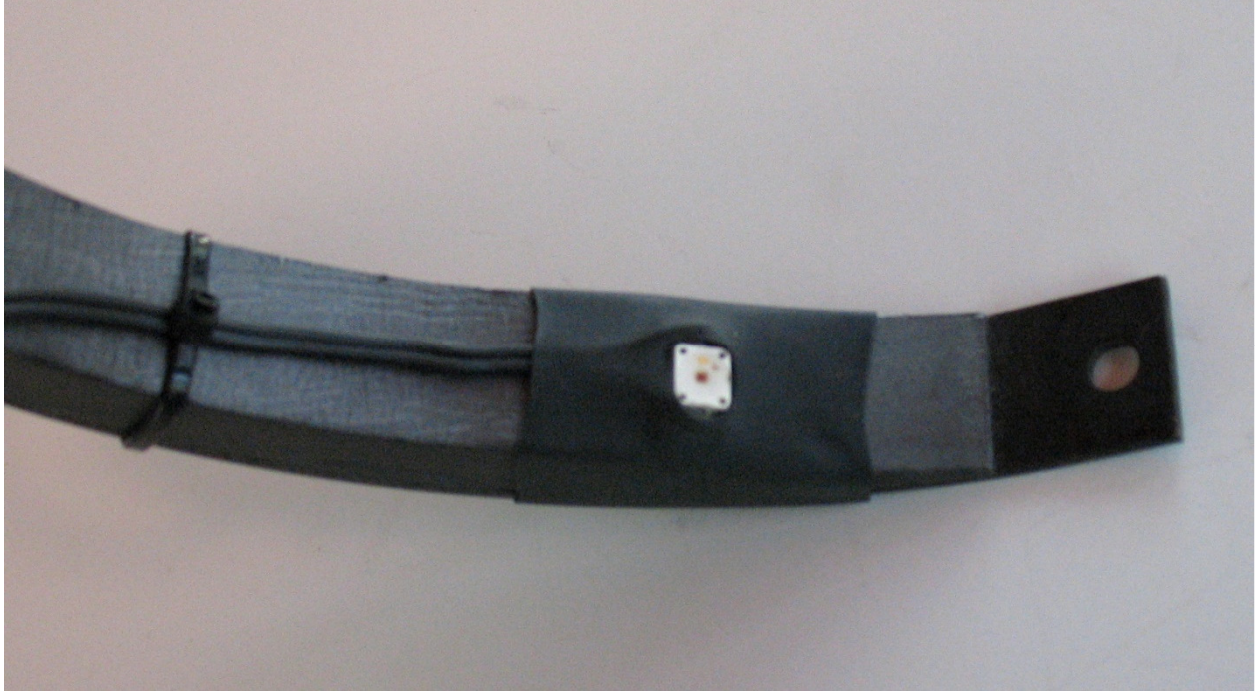
Figure 22. Flat LED in place after heat-shrinking
