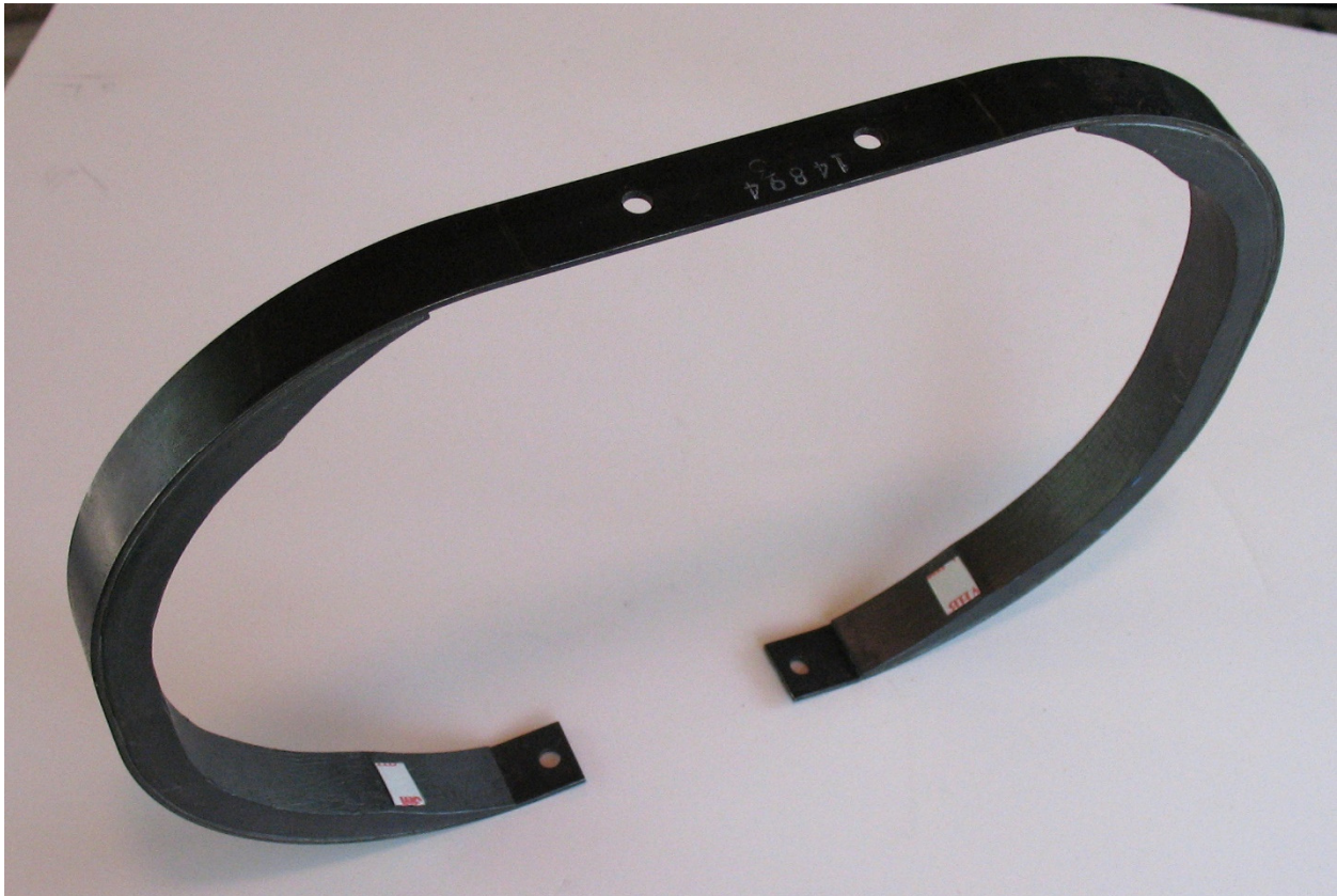
Figure 14. Rib with double-stick foam tape in place
