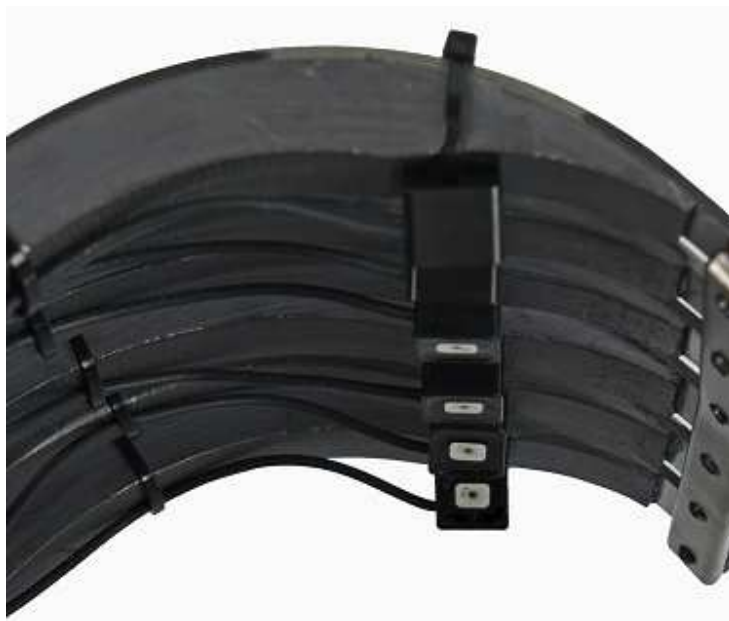
Figure 12. All six LEDs on one side of ribcage
