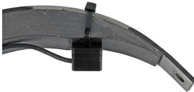
Figure 9. Putting a LED on Rib #1 (top rib) with nylon tie
