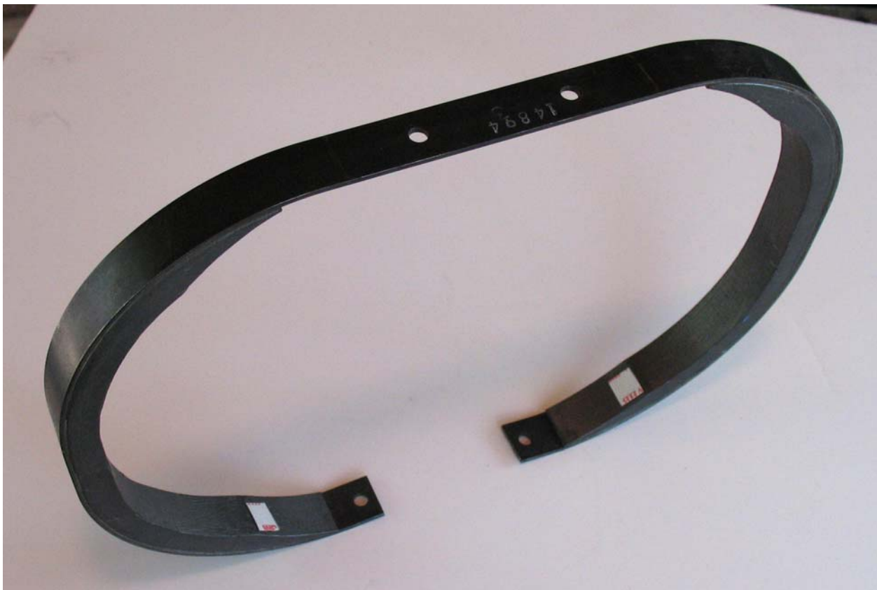
Figure 14. Rib with double-stick foam tape in place
