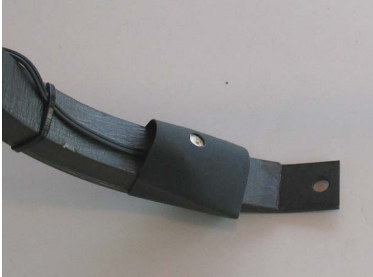
Figure 20. Heat-shrink sleeve in place over angled LED
