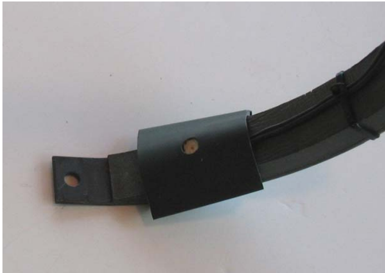
Figure 20. Heat-shrink sleeve in place over angled LED
