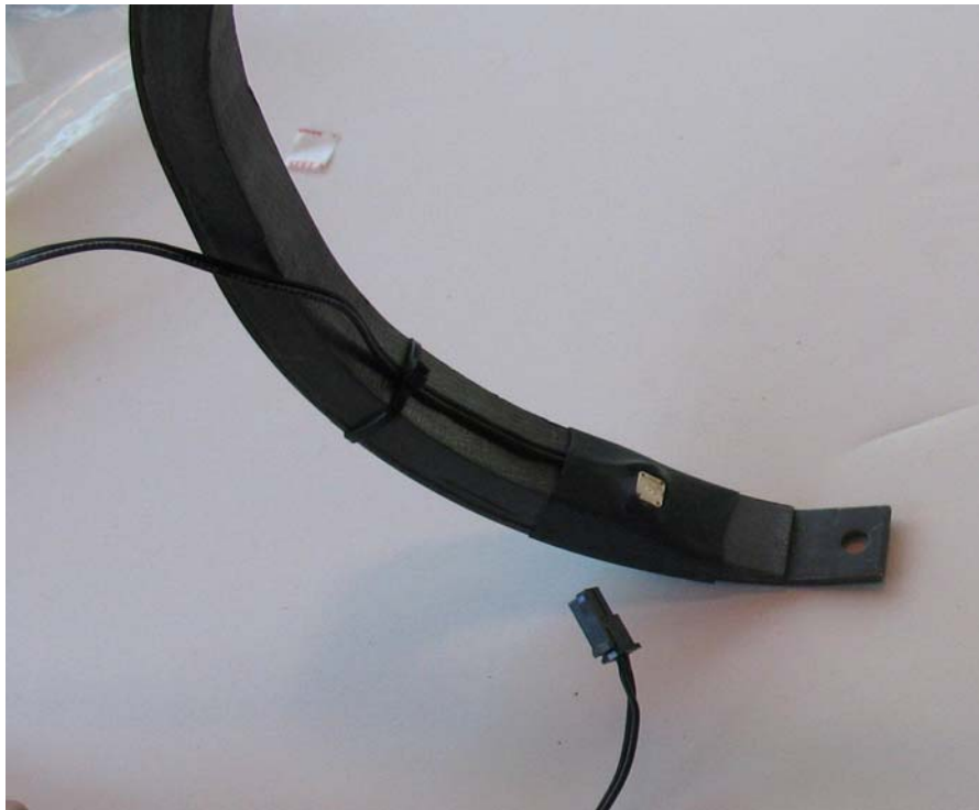
Figure 25. Angled LED and lead wire installed
