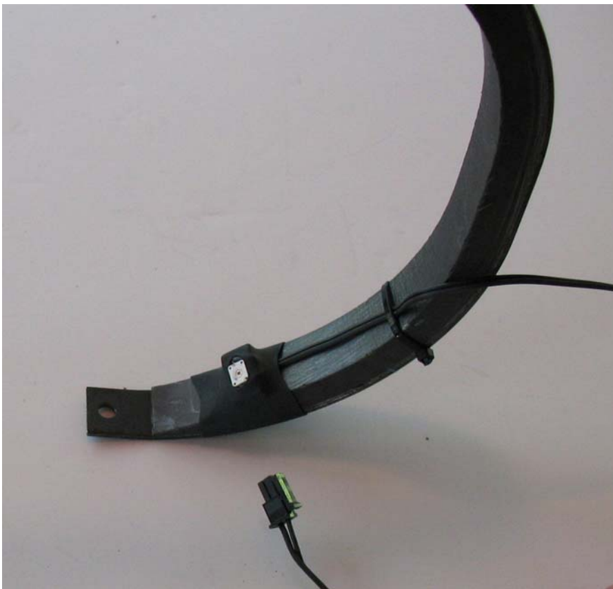
Figure 25. Angled LED and lead wire installed
