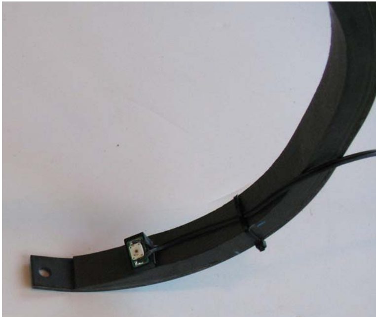
Figure 18. Angled LED in place on rib with lead wire secured by nylon tie
