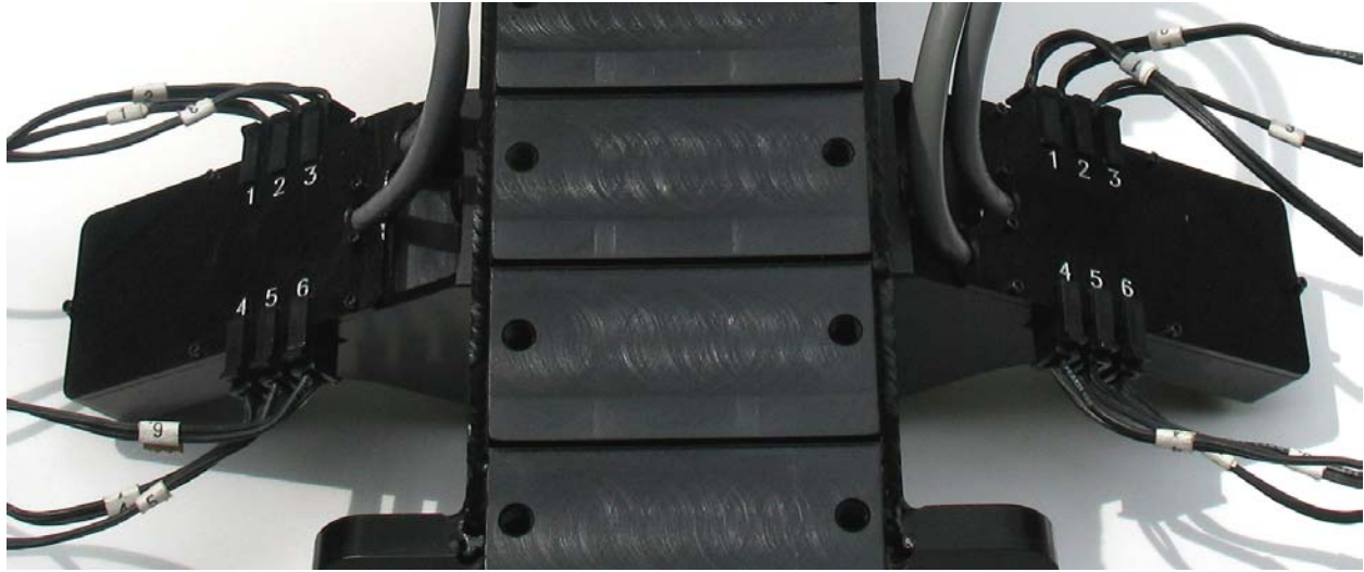
Figure B8. LED cables (lead wires) attached to connector blocks in RibEye sensor heads (rear spine view)
