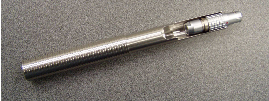
Figure 4. RibEye controller cable removal tool
