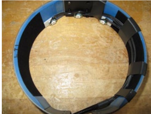
Figure 18. LEDs on thorax rib 1 of the WorldSID-50M after relocation from the centerline to the bottom edge where all the LEDs are horizontally oriented (view is looking down onto the top of the rib).
