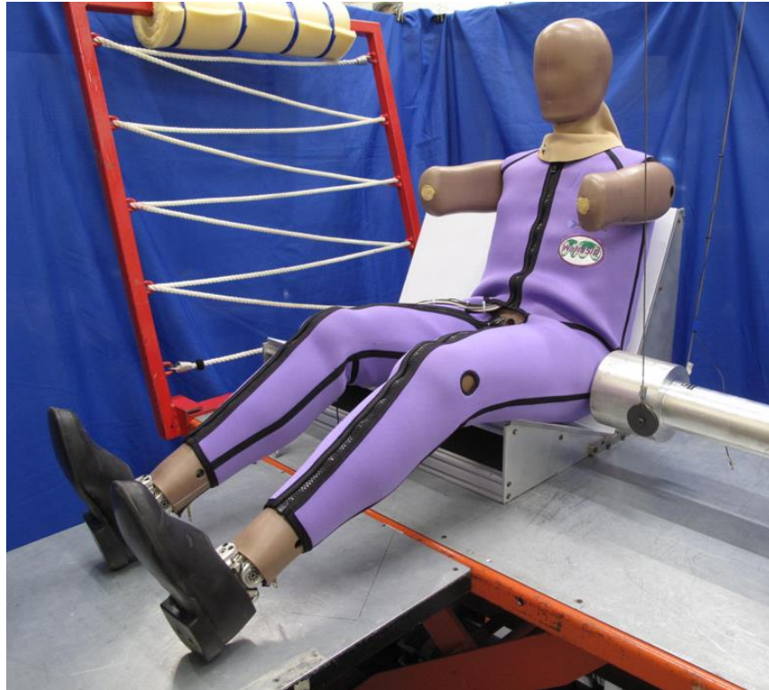
Figure 8-21. Dummy positioned for left side pelvis qualification test.
