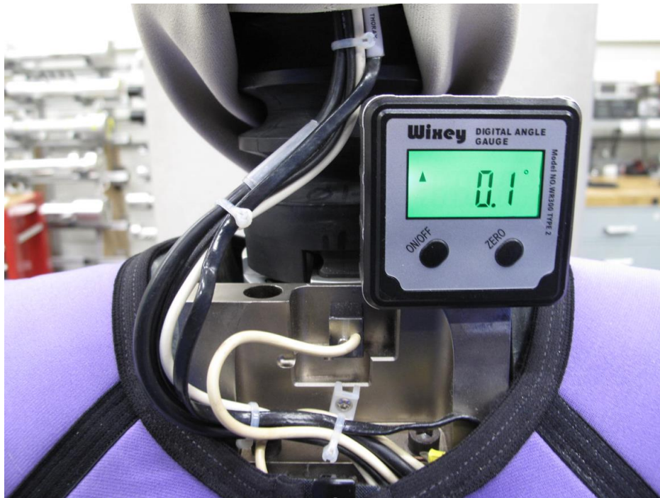
Figure 8-7. Thorax x-axis angle measurement using an inclinometer.
