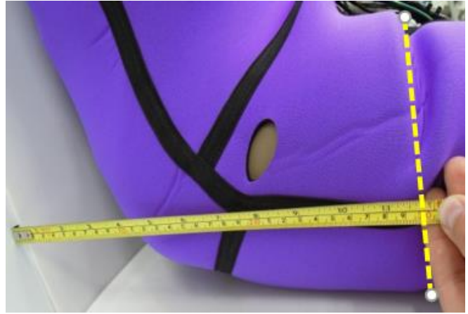
Figure 8-6. Right-side pelvis measurement.
