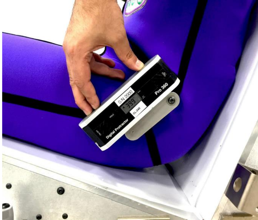
Figure 8-9. Pelvis y-axis angle measurement using H-point tool and an inclinometer.
