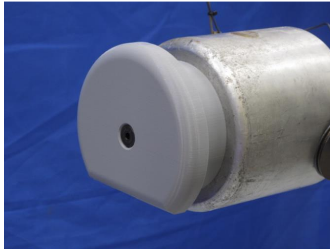
Figure 8-14. Modified impactor face attached to front of impactor.
