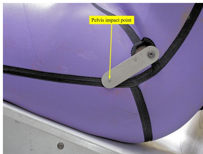
Figure 8-20. Pelvis qualification impact point at H-point.
