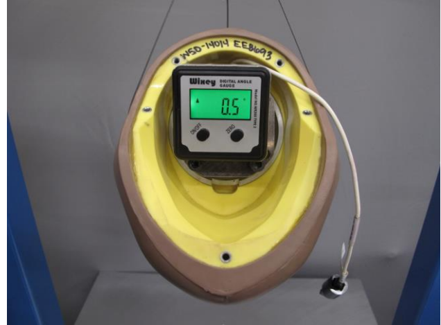
Figure 5-8. Lateral axis (y-axis) measured at the base of the load cell structural replacement.
