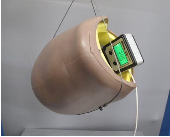
Figure 5-4. Midsagittal (x-z) plane angle measured at the base of the load cell structural replacement.
