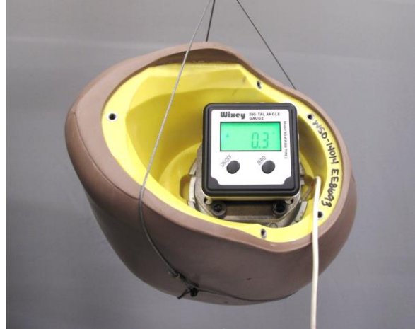
Figure 5-5. Anterior-posterior axis (x-axis) measured at the base of the load cell structural replacement.
