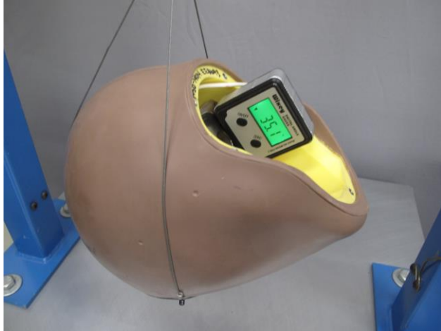
Figure 5-7. Coronal (y-z) plane angle measured at the base of the load cell structural replacement.
