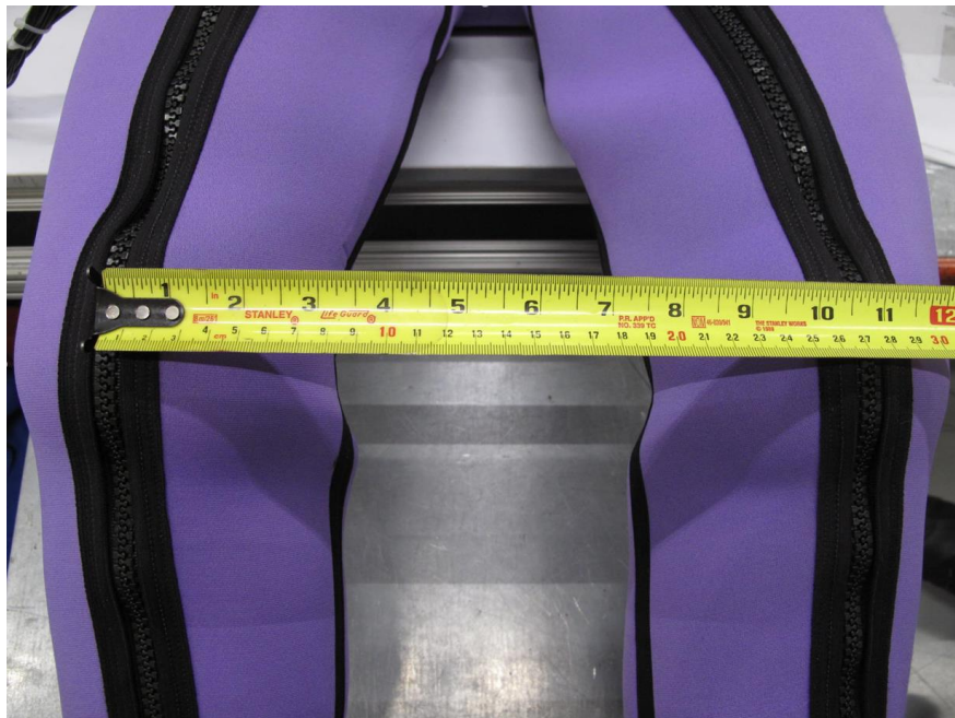
Figure 8-10. Knee centers spaced at 279 \pm 50 mm.
