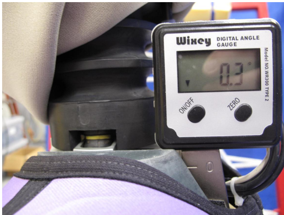
Figure 8-8. Thorax y-axis angle measurement using an inclinometer.
