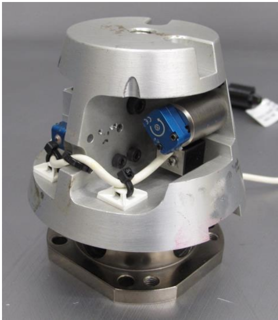
Figure 5-1. Head core and upper neck load cell structural replacement.
