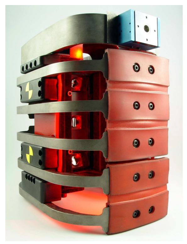
Figure 6. RibEye controller/sensor mounted in the SIDIIs thorax
