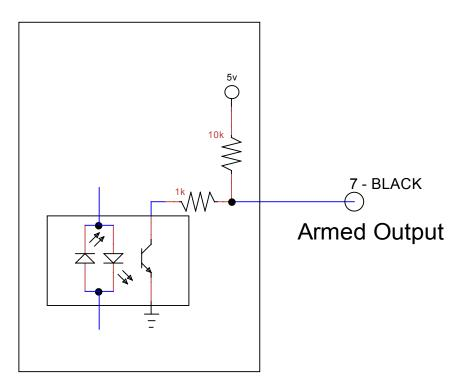
Figure B5. Armed output circuit
