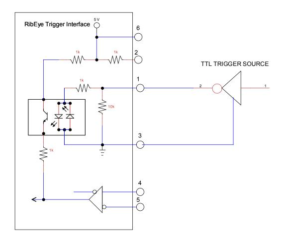
Figure B3. TTL trigger source connection
