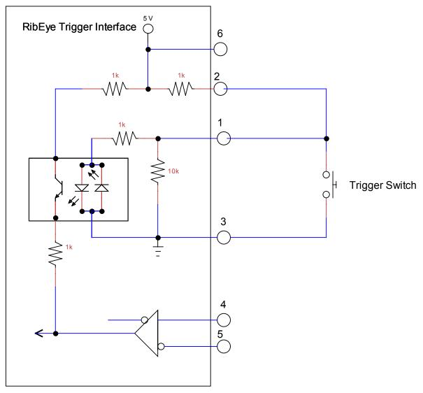
Figure B1. Trigger switch connection
