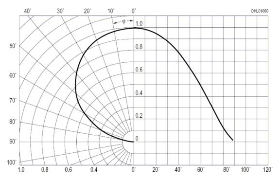
Figure 5. LED radiation pattern
