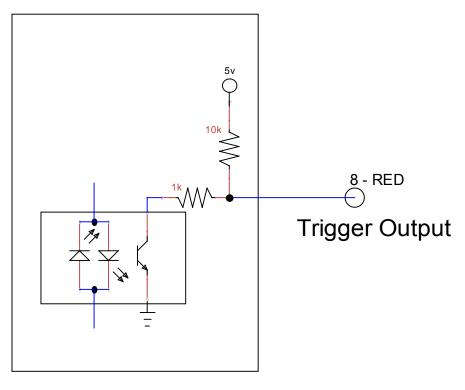
Figure B6. Trigger output circuit
