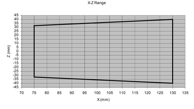
Figure A2. RibEye measurement range in X-Z plane
