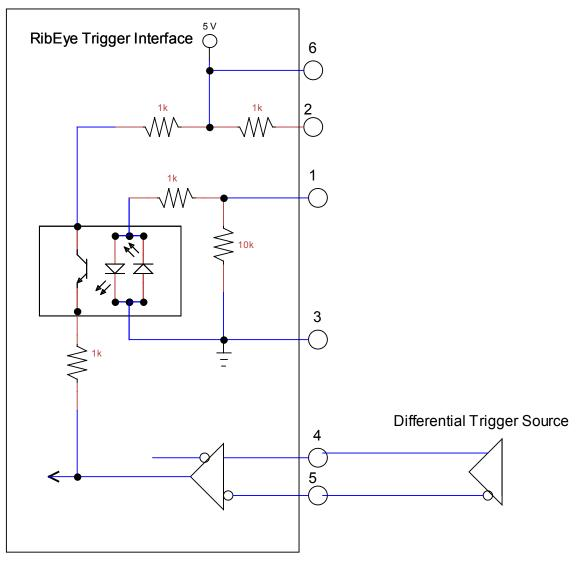
Figure B4. Differential trigger source connection
