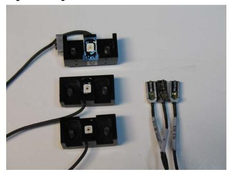
Figure 2B. Newer style LEDs for three-rib fixture
