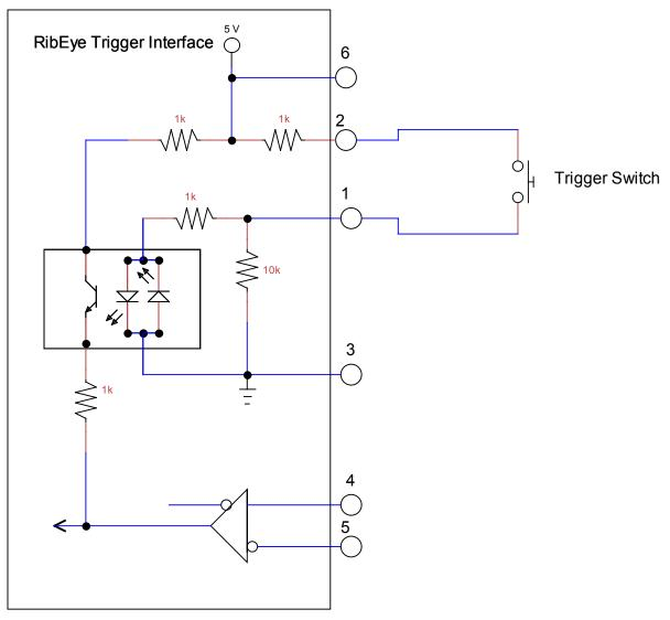
Figure B2. Alternate trigger switch connection
