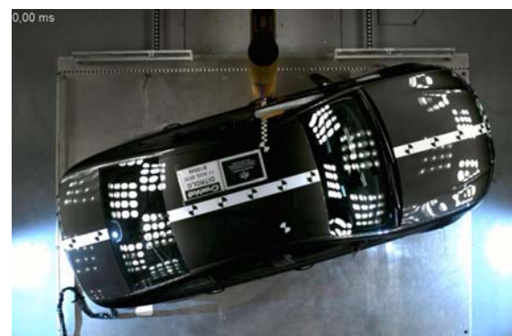
Figure 8. Overhead view of an oblique pole side impact test (Model B at time-zero).
