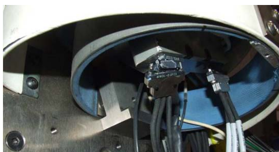
Figure 31. Damage to “RibEye” controller sensor cable connector in the oblique pole test conducted on Model B.
