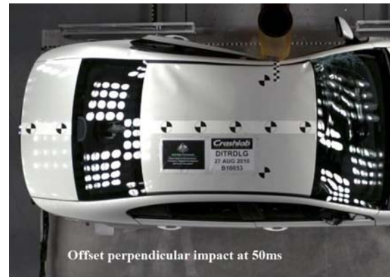
Figure 32. Overhead (plan) view of offset perpendicular impact of Model B, 50 ms after first vehicle contact with the pole.
