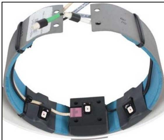
Figure 2. A WorldSID 50 th male rib fitted with three "RibEye" LEDs.
