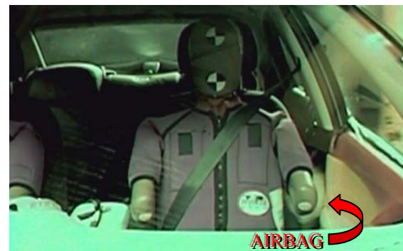
Figure 11. Model A airbag deployment near lower thorax and abdomen of WorldSID male.
