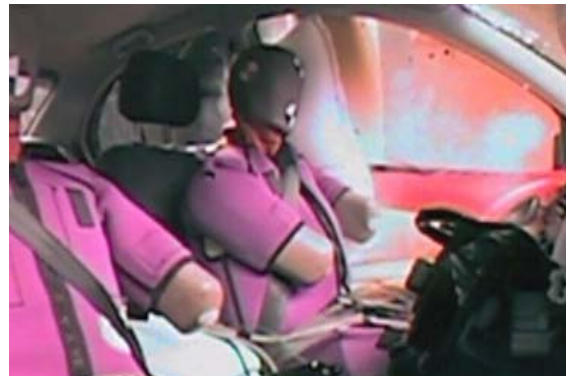
Figure 17. Side view of Model A airbag deployment, 50 ms after first vehicle contact with the pole in the oblique pole test.
