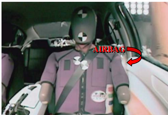
Figure 16. Model B airbag deployment near shoulder of WorldSID male.
