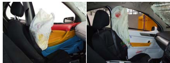
Figure 3. Deployed head/thorax combination side airbags (left: Model A; right: Model B).
