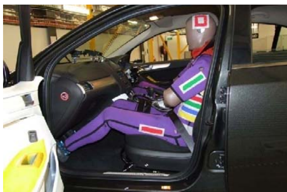
Figure 5. An example of multi-colour paint markings used to leave evidence of dummy contact during a test.
