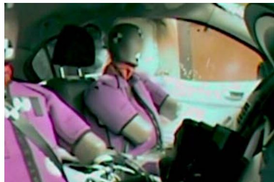
Figure 18. Side view of Model B airbag deployment, 50 ms after first vehicle contact with the pole in the oblique pole test.
