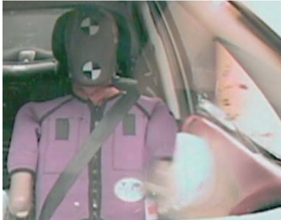
Figure 12. Model A airbag deployment 18 ms after first vehicle contact with the pole in the perpendicular test.
