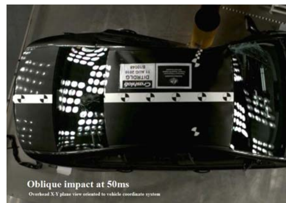
Figure 33. Overhead (plan) view of oblique impact of Model B, 50 ms after first vehicle contact with the pole (note: image has been digitally rotated 15 degrees clockwise for comparison purposes).
