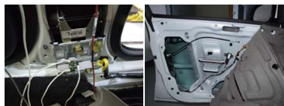
Figure 4. Model A lower b-pillar acceleration type sensor (left) and Model B door cavity pressure sensor (right).
