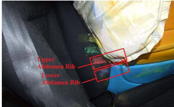
Figure 34. Struck side dummy thorax/abdomen rib to airbag and armrest interaction in the oblique pole test conducted on Model A.
