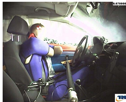
Figure 14. Comparison of driver dummy kinematics (ES-2 left, WorldSID 50M right), showing ES-2 shoulder moving forward away from ribs (shrugging).
