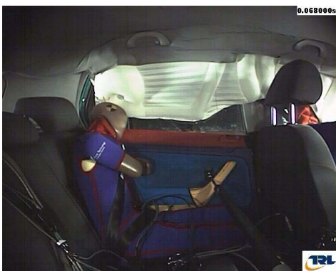
Figure 15. WorldSID 5F rear passenger showing head contact with door - head not protected by airbag.
