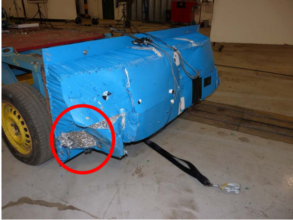
Figure 9. AE-MDB from 60 km/h Golf test showing that barrier was close to ‘bottoming out’.
