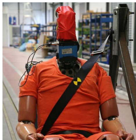
Figure 8. A camera facing down into the inside of the chest of the dummy
