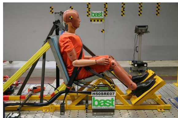
Figure 3. The test setup consisted of a rigid seat, foot rest and a standard three-point belt system.
