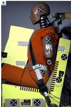
Figure 6. Static deployment test with diagonal belt only and retractor pretensioning.
