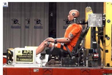
Figure 4. Generic environment, Hybrid III with rib eye sensors.
