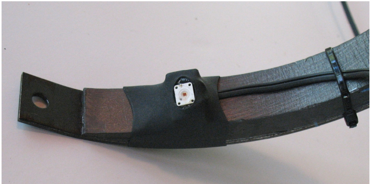
Figure 24. Angled LED in place after heat-shrinking
