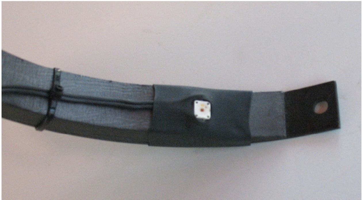
Figure 24. Angled LED in place after heat-shrinking
