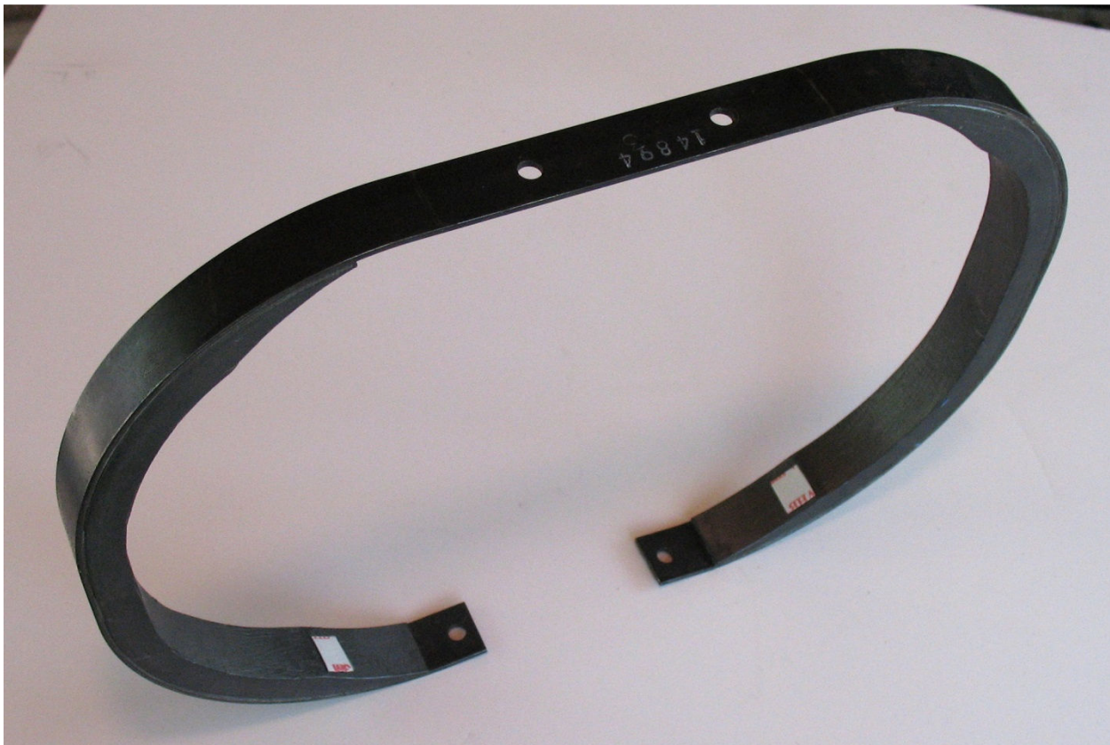
Figure 15. Rib with double-stick foam tape in place
