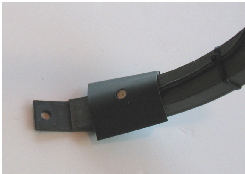
Figure 21. Heat-shrink sleeve in place over angled LED
