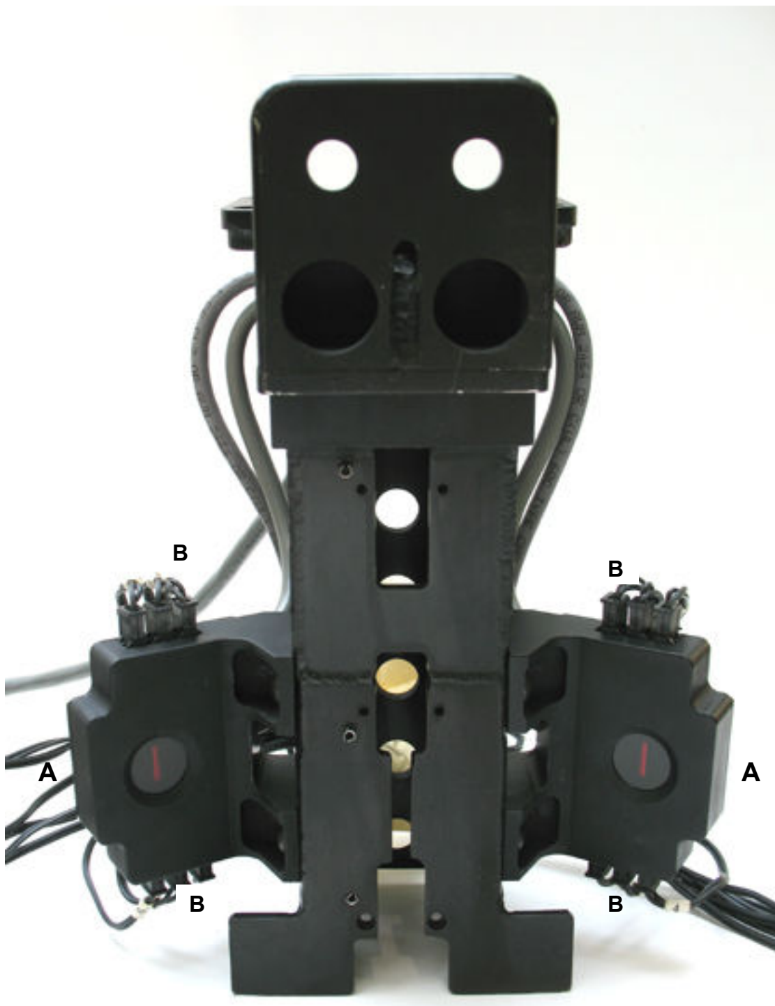
Figure 2. Front view of spine A = sensor heads; B = LED connector blocks
