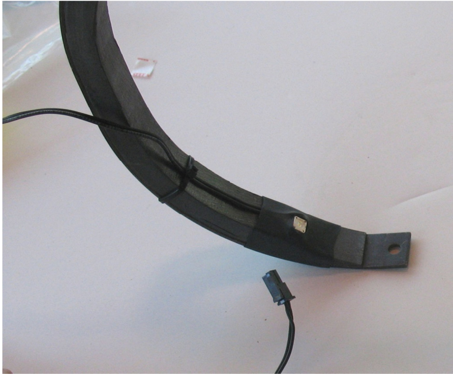
Figure 25. Flat LED and lead wire installed
