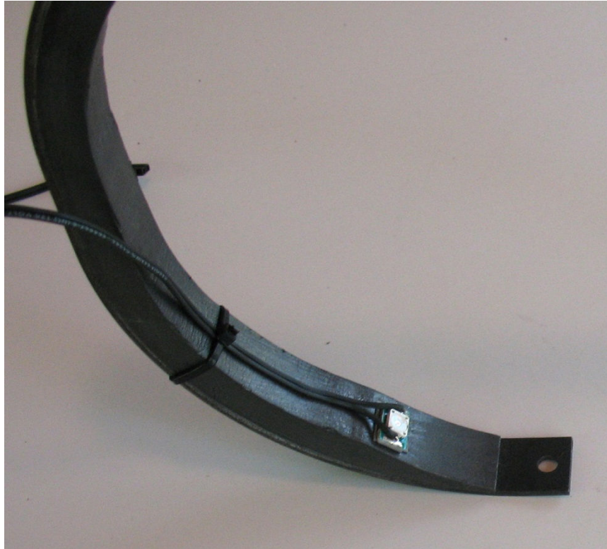
Figure 18. Flat LED in place on rib with lead wire secured by nylon tie
