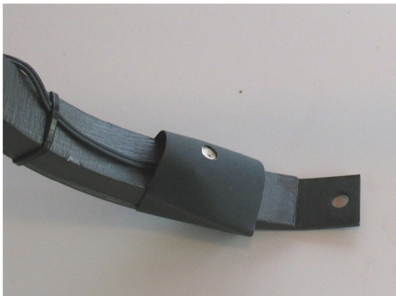
Figure 20. Heat-shrink sleeve in place over flat LED
