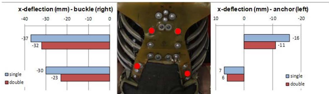
Figure 18. IR-Tracc x-deflection in the THOR dummy for single and double pretensioning
