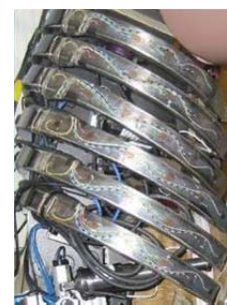
Figure 7. Ribs 2 to 7 each equipped with 6 strain gages left and right
