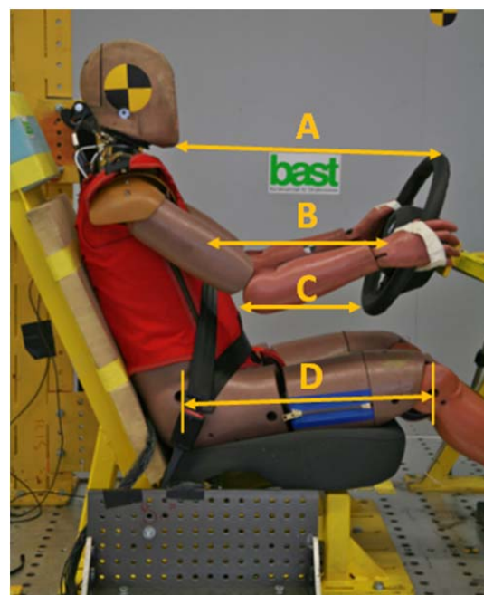
Figure 3. Positioning measurements of THOR
