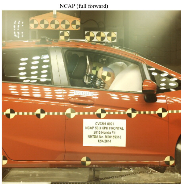
Honda Fit, test #9337, air bag deployment at 0.046 seconds
