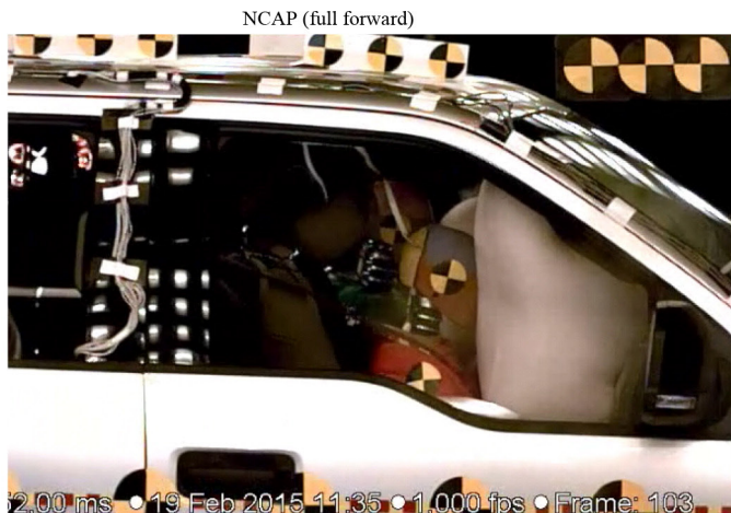
Ford F-150, test #9335, air bag deployment at 0.052 seconds
